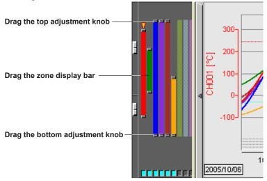
You can change the waveform display zone on the trend display screen by clicking the edit zone icon on the tool bar or by selecting [Y-Axis] - [Edit Zone] in the menu bar.
