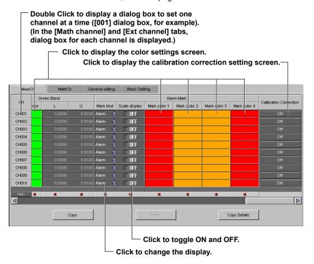
Enter external input channel settings in the same manner as those of the measurement channel items. Also note that this measurement channel setting screen is only one example; your actual screen may vary.
