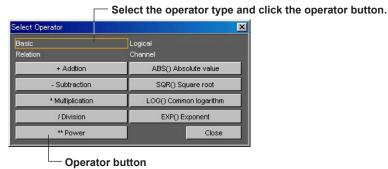
The items of the [Math] tab can be set for each channel. The items set here are the same as the ones in the [Math] tab of the Hardware Configurator. For details, see the page corresponding to the item.
