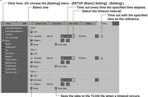
You can set three types of timers to be used in the statistical computation. You can save the data to a TLOG file or reset the computation when the specified timeout interval elapses. This function is available only if the Computation function is installed. For details about the types of timers and various settings, refer to the *CX User's Manual (IM 04L31A01-01E or IM 04L31A01-03E)*.
