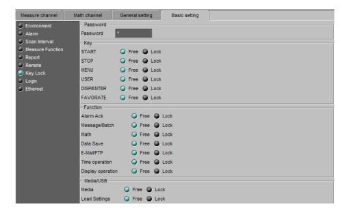
Enabled when [Key Security] is set to [Keylock] under [Environment] - [Detail Setting] in the [Basic Setting] tab.
