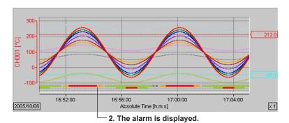
The alarm conditions of alarm 1 to 4 are displayed in the alarm display area.
