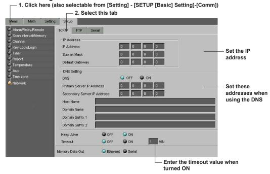
In the case of a CONFIG file, the IP address cannot be configured. When communicating with the DX100/DX200/MV100/MV200 via Ethernet, the IP address, subnet mask, and default gateway must be set on the DX100/DX200/MV100/MV200 beforehand.
