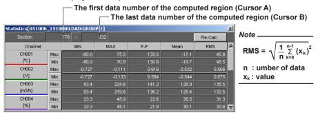
The minimum value, maximum value, P-P, mean, and rms value for each waveform in the range specified by Cursors A and B are computed and displayed. If the cursor is not displayed, the computation is performed over the entire data.
