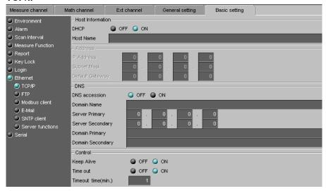
Set the IP address to a fixed IP address or obtain it automatically (DHCP). Consult with your network administrator for the network parameters such as the IP address, subnet mask, default gateway, and DNS.
