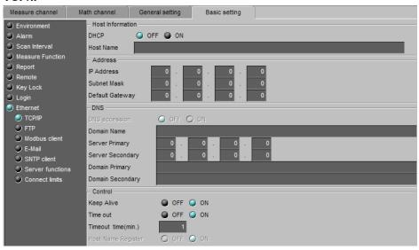
Set the IP address to a fixed IP address or obtain it automatically (DHCP). Consult with your network administrator for the network parameters such as the IP address, subnet mask, default gateway, and DNS.
