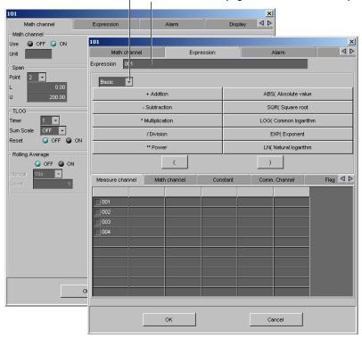
The items in the math channel tab can be configured for each channel. The items that are configured are the same as those configured on the spreadsheet. For details, see the page corresponding to the item.
