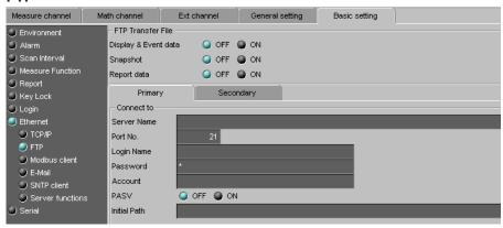
The data files are automatically transferred to the FTP destination.
