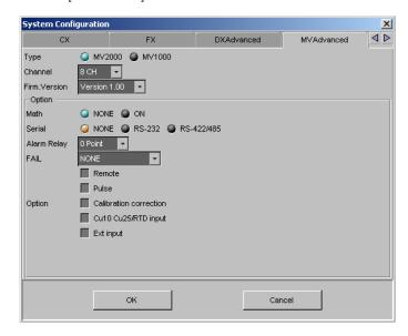
**2.** Enter all settings on the [MVAdvanced] tab, then click the [OK] button. The MV1000/MV2000 setting screen in displayed.
