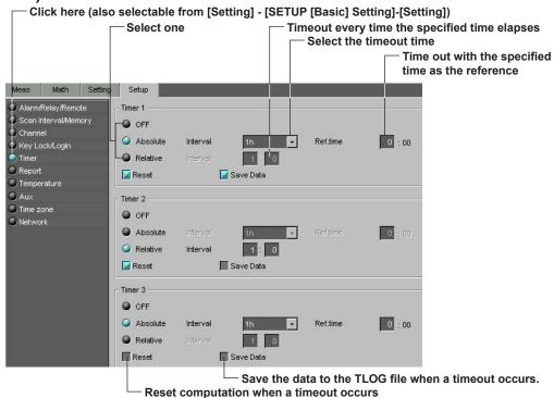
You can set three types of timers to be used in the statistical computation. You can have the data saved to a TLOG file or reset the computation when the specified timeout time elapses.
