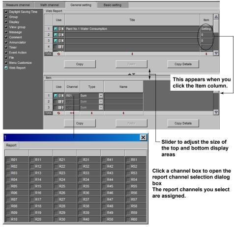
These settings affect how report data in the internal memory is displayed on the operator and monitor pages. You can create 10 report layouts. You can register up to 10 items to display in each layout.
