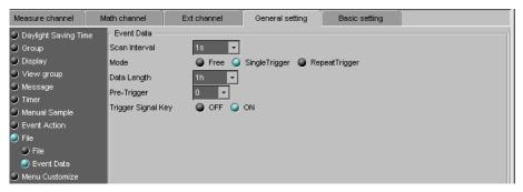
Event related settings are enabled when [Data Kind] is set to [E+D] or [Event] in [Basic Environment] under [Environment] in the [Basic Setting] tab.
