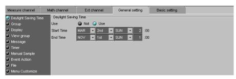
On/Off To switch between summer time and standard time, select [On].
